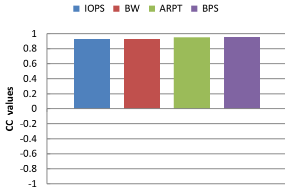
Figure 4. The normalized CC values of IOPS, bandwidth (BW), average response time (ARPT), and BPS.
