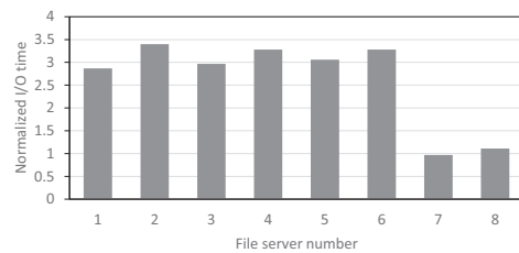
(a) I/O time of each server under a fixed I/O pattern and stripe size
